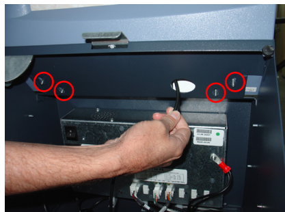
Figure 2. Feed topper power cable through cabinet access hole.
