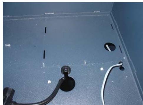
Figure 24. Power supply and dispenser data cable removed from cabinet.
