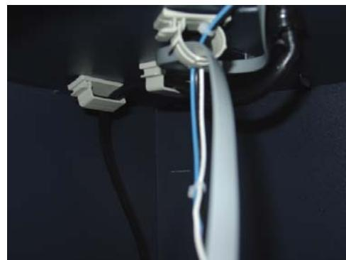
Figure 27. Route cables through clip.
