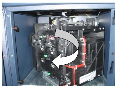
Figure 2. Rotate dispenser clockwise.
