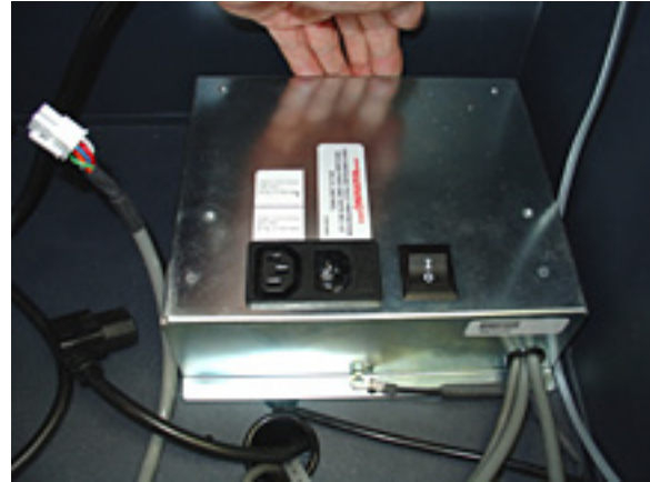
Slide the single power supply forward and lift it from the cabinet top enclosure
