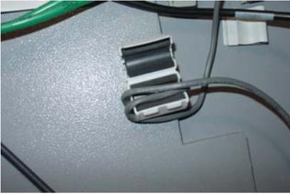
*Figure 17. Install cable in ferrite.*
