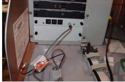
*Figure 18. Connect cable to Tri-Port module.*
