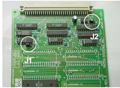
Figure 15. Memory Expansion module J1 and J2 jumper location (pins 1 and 2).
