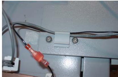
Figure 12. Install flat clip and secure cable.
