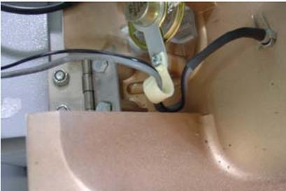
Figure 11. Install clip and route cable.
