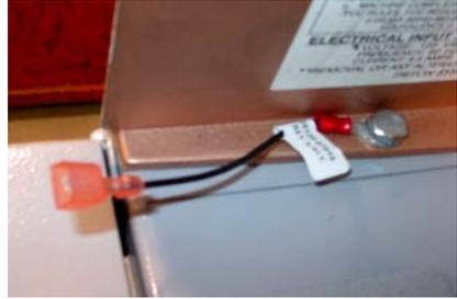
Figure 10. Install ground wire adapter.
