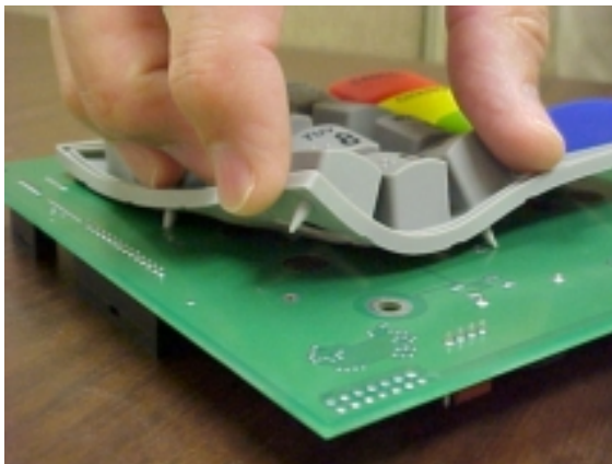
FIGURE 3c. ALIGNING CLEATS WITH HOLES IN SPED BOARD.
