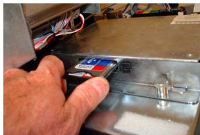
Figure 2. Insert into PCMCIA slot.
