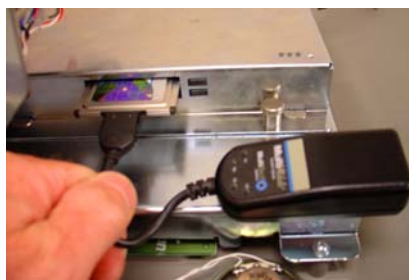
Figure 2. Remove PCMCIA modem card and adapter.
