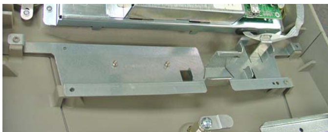
Figure 3. Install modem mounting bracket.
