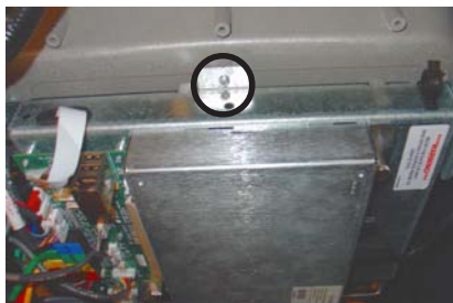
Figure 2. Secure bracket to screw shown.
