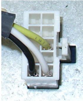
The TDM dispenser DC power cable connection (10-pin connector) at the dual power supply
