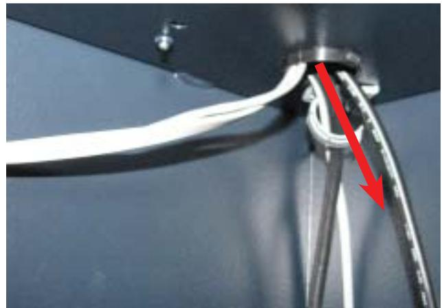
7. Route the dispenser communication cable down the front of the dispenser tray, through the quick release cable clip and under the tray. Pull all excess cable up from behind the tray as shown.
