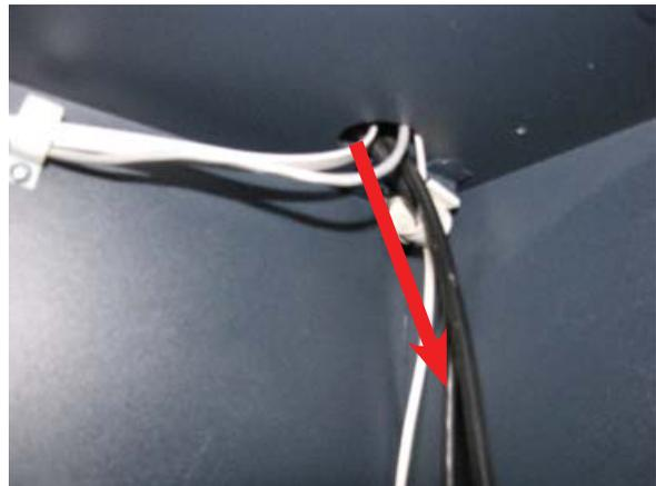
7. Route the dispenser communication cable down in front of the dispenser tray, through the quick release cable clip, under the tray and up from behind the tray as shown.
