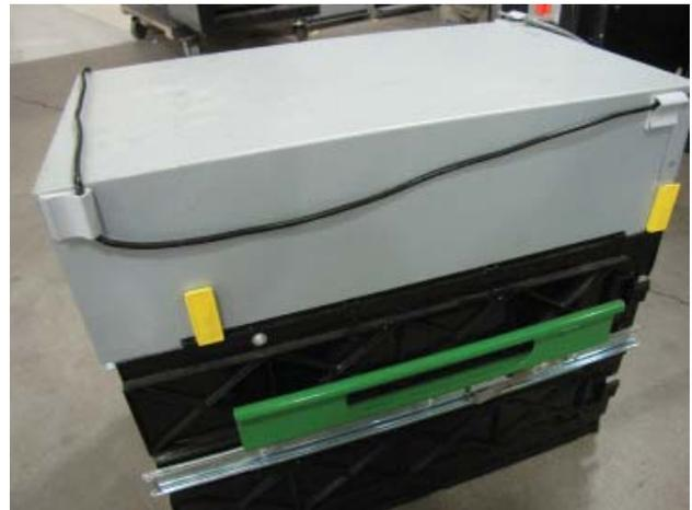
16. Route the Dispenser Communication Cable across the top of the dispenser, through the cable clip on the left side of the dispenser and plug it into the dispenser as shown.
