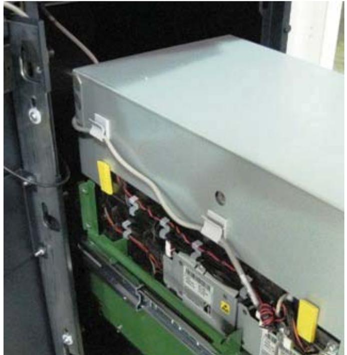
16. Route the Dispenser data cable from the security module assembly through the two cable clips on the right side of the NMD50 dispenser as shown.
