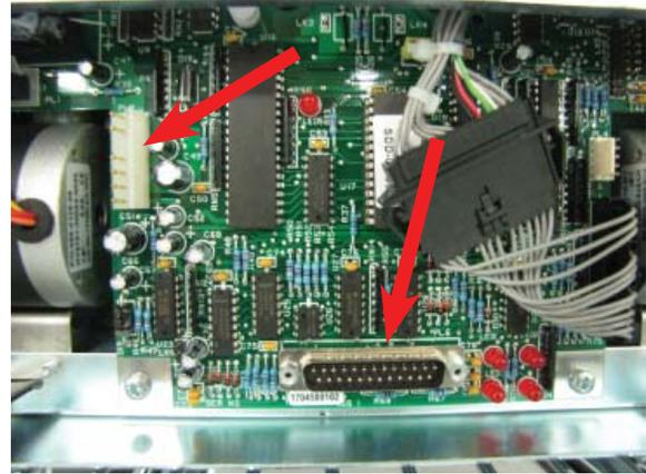
15. Route the security module communication and security module power cable around the unit's main power cable and over the power supply (red arrows). Plug the power cable into the power supply.
