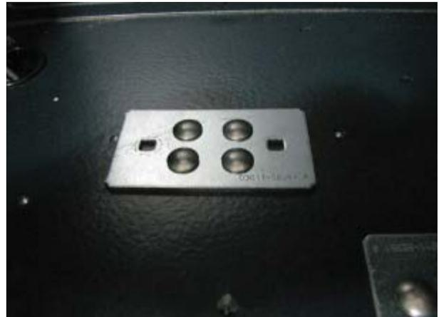
9. Install the lower closeout bracket on the bolts in the lower cabinet. Using the 7/16" hollow shaft but driver, install the nuts on the bolts; 6 nuts on the nut and 4 bolts in the middle. While tightening, ensure the bolts and bracket are sitting flat in the upper cabinet.
