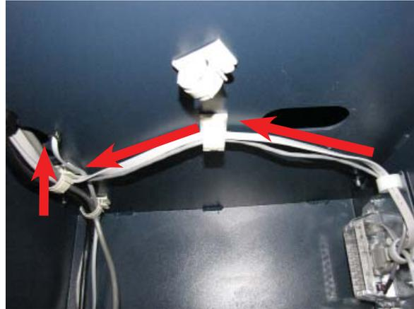
6. Obtain the dispenser power cable. Plug the power cable into the unit's power supply in the upper portion of the cabinet. Route the cable through the left hole opening into the lower cabinet.
