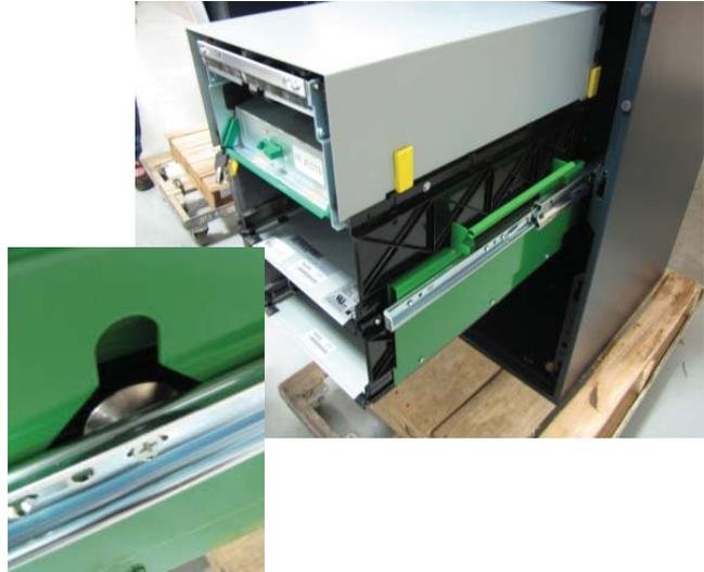
12. Route the ground wire around to the front of the dispenser. Plug the ground wire onto the quick connect as shown.
