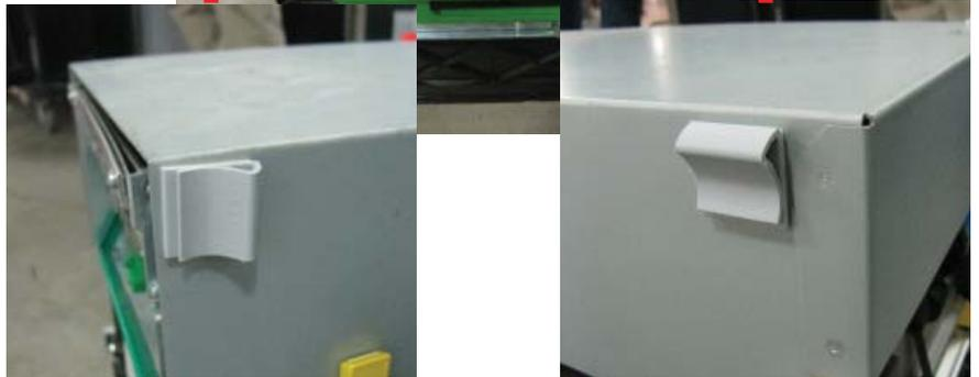
10. Peel the paper backing off one Panduit Adhesive Cable Clip and adhere it to the front left side of the NMD50 dispenser. Note the orientation of the clips in the pictures.
