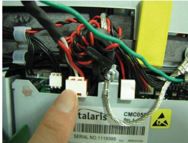
18. Tuck the ground wire under the clip on the side of the dispenser. Route the power cable through the two cable clips along the left side of the dispenser. Route the cable around to the rear of the dispenser and through the cable clip on the back left side of the NMD50.
