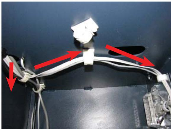
6. Obtain the dispenser power cable. Plug the power cable into the unit's power supply in the upper portion of the cabinet. Route the cable through the left hole opening into the lower cabinet. Route the cable through the two left side cable clips.
