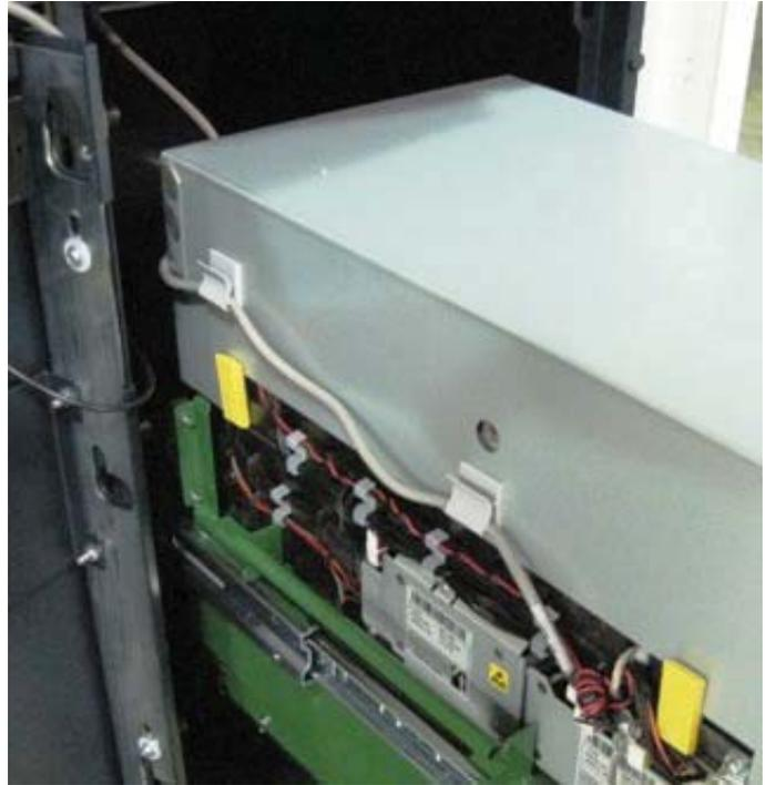
15. Route the Dispenser data cable from the security module assembly through the two cable clips on the right side of the NMD50 dispenser as shown.
