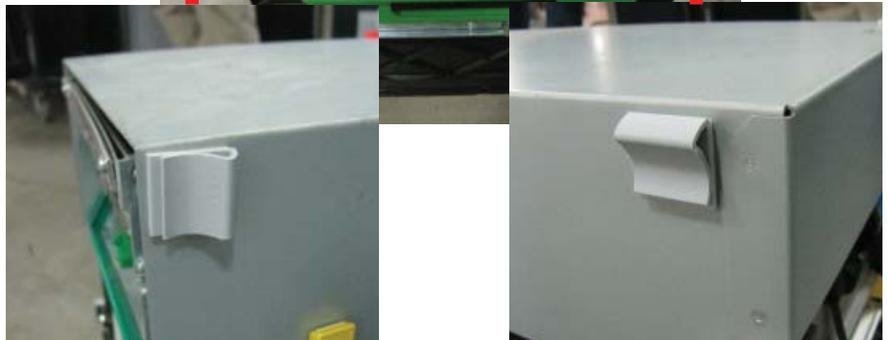
14. Peel the paper backing off one Panduit Adhesive Cable Clip and adhere it to the front left side of the NMD50 dispenser. Note the orientation of the clips in the pictures.
