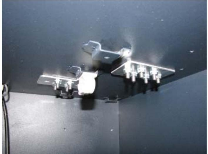
9. With the dispenser still removed from the unit, peel the paper backing off one Panduit Adhesive Cable Clip and adhere it to the back right side of the NMD50 dispenser. Peel the paper backing off another Panduit Adhesive Cable Clip and adhere it to the front right side of the NMD50 dispenser. Note the orientation of the clips in the pictures.
