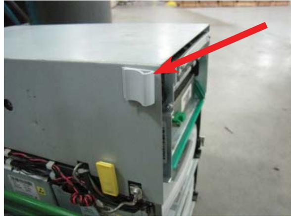
15. Remove the cassettes from the NMD50 if installed. Pull both slides out fully and ensure they lock into place. Set the dispenser into position ensuring the posts on the rails sit securely in the handle's notches. Reinstall the cassettes.
