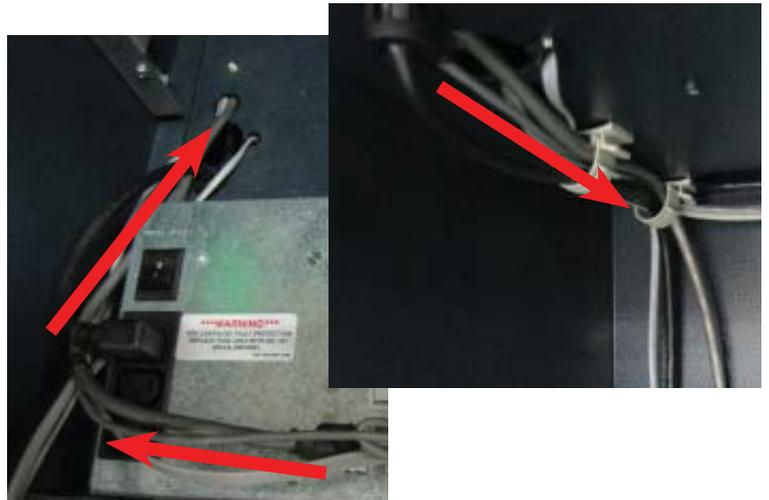
7. Loop the SDD dispenser communication cable back on itself twice to condense the length of the cable to match the length of the dispenser power cable. TY Wrap the two cables together in two spots as shown. Cut off the excess TY Wraps.
