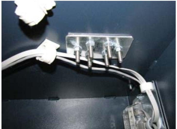
11. Plug the cables into the back of the SDD dispenser and tighten the thumbscrews on the communication cable to secure it. Reinstall the dispenser into the unit.
