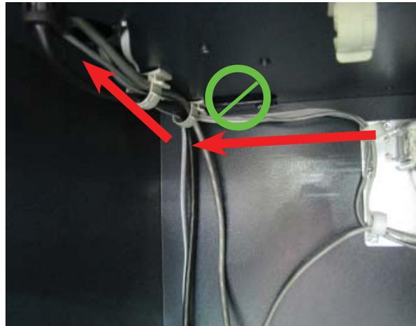
6. Obtain the dispenser power cable. Plug the power cable into the unit's power supply in the upper portion of the cabinet. Route the cable through the left hole opening into the lower cabinet. Route the cable through the two left side cable clips.
