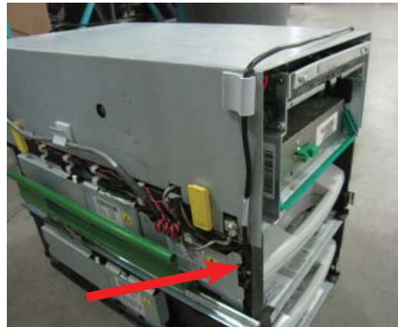
18. In the upper cabinet, route all the cables through the cable clip previously installed. Route the cables under the bracket as shown.
