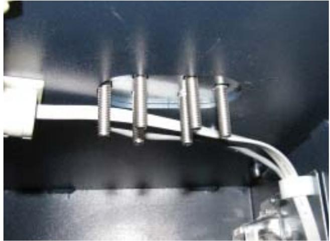
9. Install the second closeout bracket on the bolts in the lower cabinet. Using the 7/16" hollow shaft nut driver, install the 6 hex nuts on the bolts. While tightening, ensure the bolts and bracket are sitting flat in the upper cabinet.
