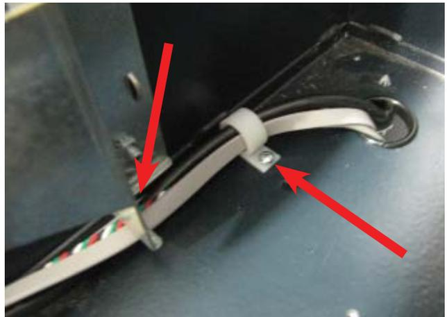
19. Route the security module communication and security module power cable around the unit's main power cable and over the power supply (red arrows). Plug the power cable into the power supply.
