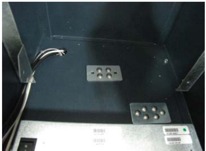
8. Install the lower closeout bracket on the 6 bolts on the right opening. Using the 7/16" hollow shaft but driver, install 6 hex nuts on the bolts. Install the second closeout bracket onto the 4 bolts on the middle opening. Install 4 hex nuts on the bolts. While tightening, ensure the bolts and brackets are sitting flat in the upper cabinet.
