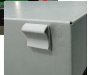
11. Peel the paper backing off one Panduit Adhesive Cable Clip and adhere it to the front left side of the NMD50 dispenser. Note the orientation of the clip in the picture.
