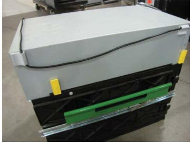
17. Route the Dispenser Communication Cable across the top of the dispenser, through the cable clip on the left side of the dispenser and plug it into the dispenser as shown.
