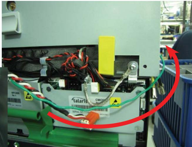
14. Plug the Dispenser Power Cable into the side of the NMD50 as shown.
