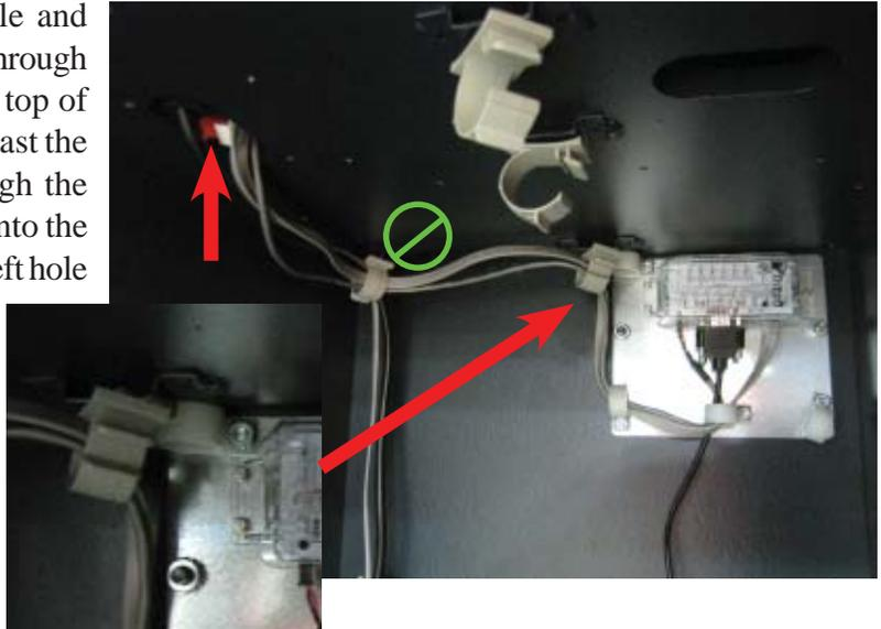
7. Obtain the dispenser power cable. Plug the power cable into the unit's power supply in the upper portion of the cabinet. Route the cable through the anti-phishing bracket and the left hole opening into the lower cabinet.
