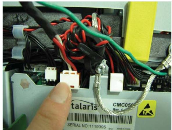
14. Tuck the ground wire under the clip on the side of the dispenser. Route the power cable through the two cable clips along the left side of the dispenser. Route the cable around to the rear of the dispenser and through the cable clip on the back left side of the NMD50.
