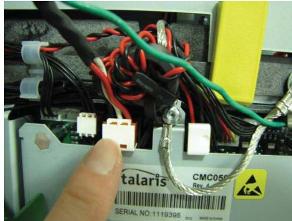
15. Tuck the ground wire under the clip on the side of the dispenser. Route the power cable through the two cable clips along the left side of the dispenser. Route the cable around to the rear of the dispenser and through the cable clip on the back left side of the NMD50.
