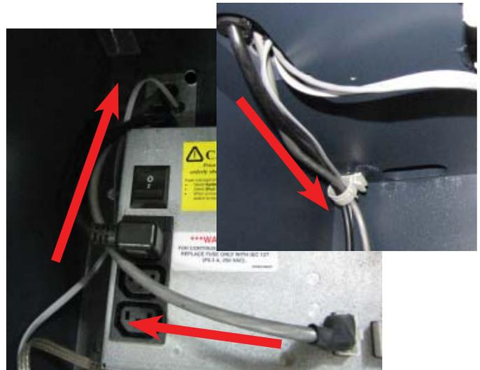
8. Loop the SDD dispenser communication cable back on itself twice to condense the length of the cable to match the length of the dispenser power cable. TY Wrap the two cables together in two spots as shown. Cut off the excess TY Wraps.
