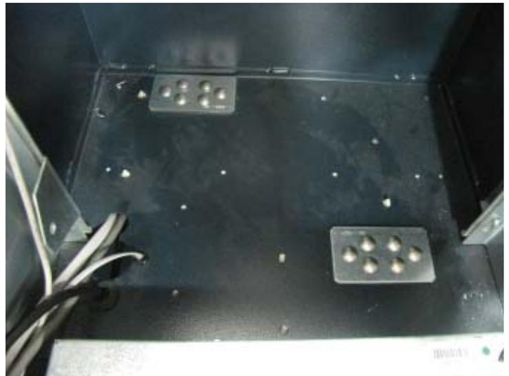
8. Ensure the bolts are not intertwined in the cables in the lower cabinet.
