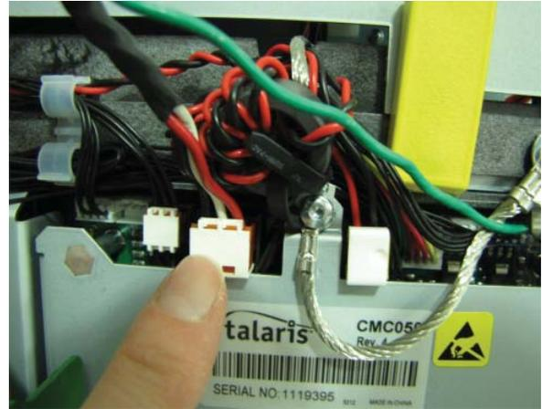
18. Tuck the ground wire under the clip on the side of the dispenser. Route the power cable through the two cable clips along the left side of the dispenser. Route the cable around to the rear of the dispenser and through the cable clip on the back left side of the NMD50.
