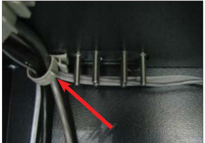
10. Install the lower close out bracket on the bolts. Using the 7/16" hollow shaft nut driver, install 6 hex nuts on the bolts. While tightening, ensure the bolts and bracket are sitting flat in the upper cabinet.
