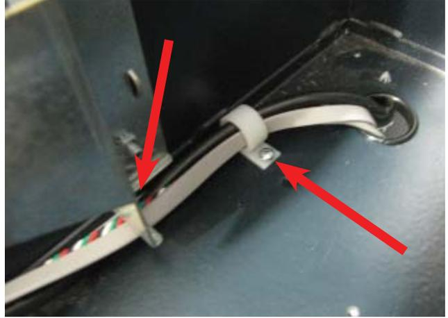
18. Loop the security module power cable back on itself to condense the length of the cable. TY Wrap the cable and cut off the excess.
