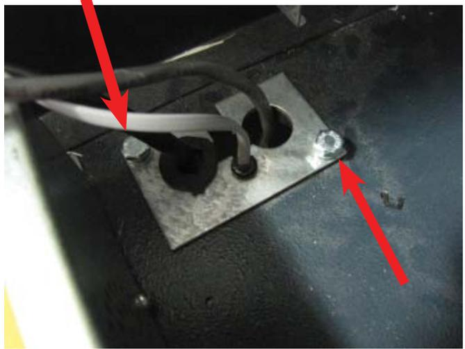
6. Route the security module power cable and security module communications cable through the rear upper middle cable clip on the top of the vault. Continue routing the cables past the back opening (green circle) and through the upper left cable clip. Route the cables into the upper portion of the cabinet through the left hole opening and the anti-phishing bracket.
