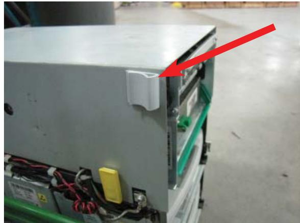
12. Remove the cassettes from the NMD50 if installed. Pull both slides out fully and ensure they lock into place. Set the dispenser into position ensuring the posts on the rails sit securely in the handle's notches. Reinstall the cassettes.
