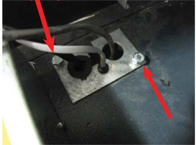
6. Route the security module power cable and security module communications cable through the upper middle back two clips. Route the cables into the upper portion of the cabinet through the left front hole opening and the anti-phishing bracket as shown.
