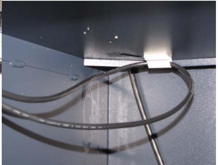
7. The data cable then comes back over the front of the Mini Mech tray and plugs into the Mini Mech.
