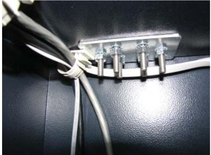
12. Install the second lower closeout bracket on the bolts in the lower cabinet. Using the 7/16" hollow shaft nut driver, install the 6 hex nuts on the bolts. While tightening, ensure the bolts and bracket are sitting flat in the upper cabinet.
