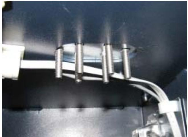
10. Install the second closeout bracket on the bolts in the lower cabinet. Using the 7/16" hollow shaft nut driver, install the 6 hex nuts on the bolts. While tightening, ensure the bolts and bracket are sitting flat in the upper cabinet.
