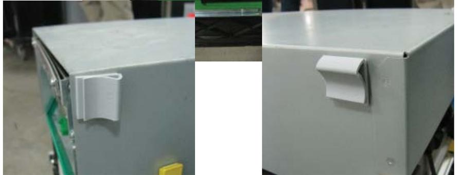
11. Peel the paper backing off one Panduit Adhesive Cable Clip and adhere it to the front left side of the NMD50 dispenser. Note the orientation of the clips in the pictures.
