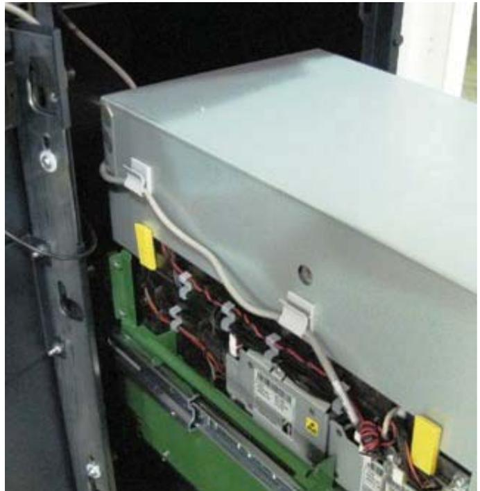
19. Route the Dispenser data cable from the security module assembly through the two cable clips on the right side of the NMD50 dispenser as shown.
