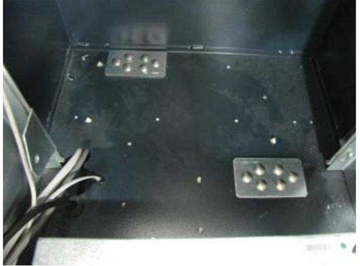
9. Ensure the bolts are not intertwined in the cables in the lower cabinet.
