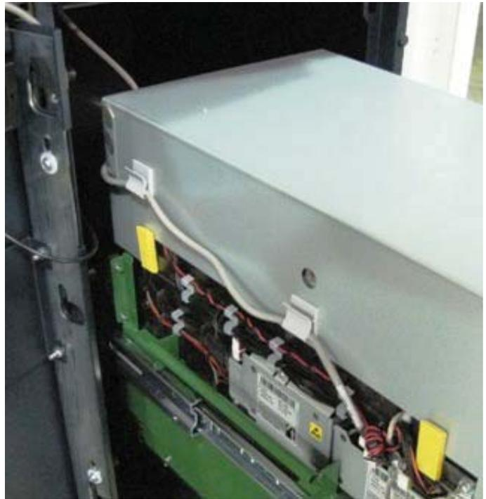
19. Route the Dispenser data cable from the security module assembly through the two cable clips on the right side of the NMD50 dispenser as shown.
