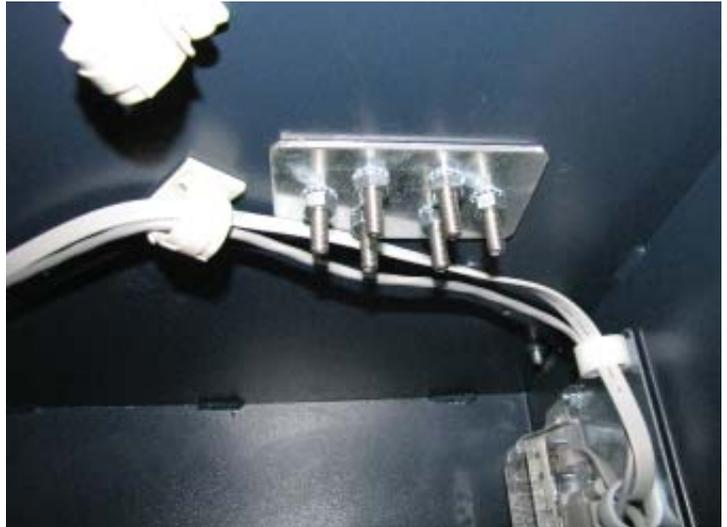
10. With the dispenser still removed from the unit, peel the paper backing off one Panduit Adhesive Cable Clip and adhere it to the back right side of the NMD50 dispenser. Peel the paper backing off another Panduit Adhesive Cable Clip and adhere it to the front right side of the NMD50 dispenser. Note the orientation of the clips in the pictures.
