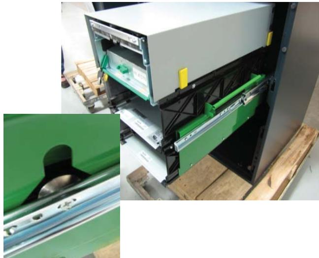
13. Route the ground wire around to the front of the dispenser. Plug the ground wire onto the quick connect as shown.
