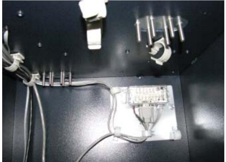
9. Remove the cable clip in the rear left corner of the lower cabinet for easier installation of the closeout bracket.
