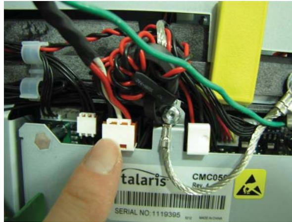
15. Tuck the ground wire under the clip on the side of the dispenser. Route the power cable through the two cable clips along the left side of the dispenser. Route the cable around to the rear of the dispenser and through the cable clip on the back left side of the NMD50.
