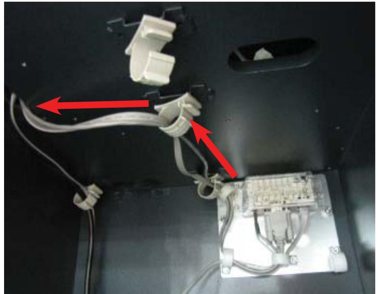
7. Obtain the dispenser power cable. Plug the power cable into the unit's power supply in the upper portion of the cabinet. Route the cable through the anti-fishing bracket and the left hole opening into the vault. Route the dispenser power cable through the rear left cable clip as shown.
