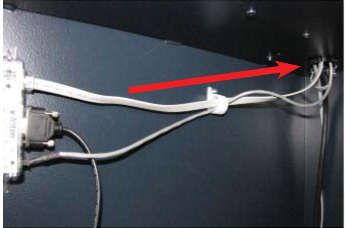
6. Obtain the dispenser power cable. Plug the power cable into the unit's power supply in the upper portion of the cabinet. Route the cable through the left hole opening into the lower cabinet.
