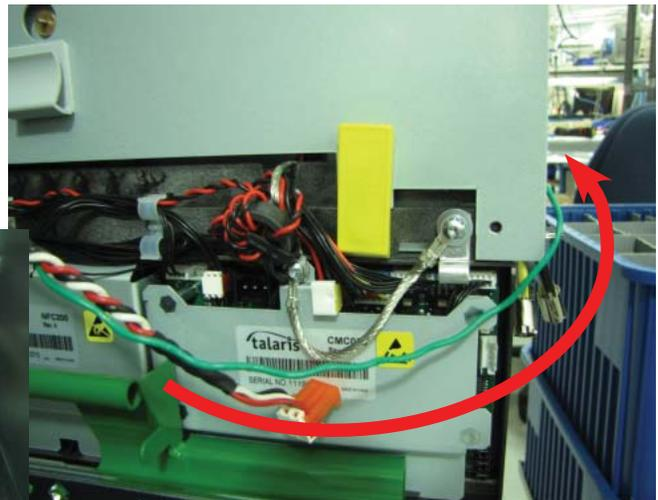
13. Plug the Dispenser Power Cable into the side of the NMD50 as shown.
