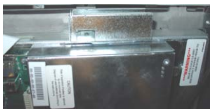
Figure 3. Modem bracket mounted.
