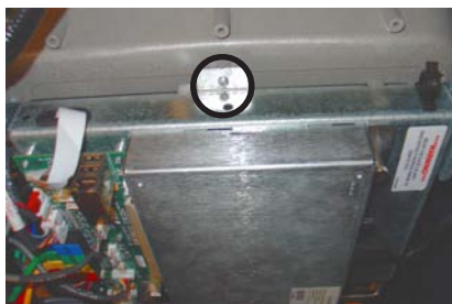
Figure 2. Secure bracket to screw shown.
