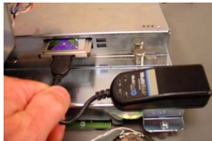
Figure 2. Remove PCMCIA modem card and adapter.
