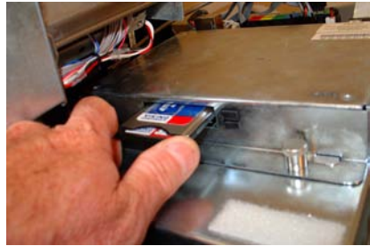
Figure 2. Insert into PCMCIA slot.
