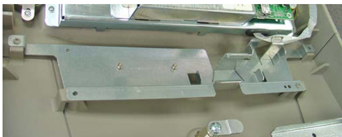
Figure 3. Install modem mounting bracket.
