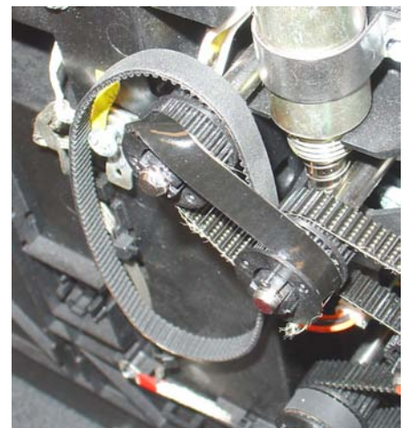
Roll Upper belt to install on pulleys.
